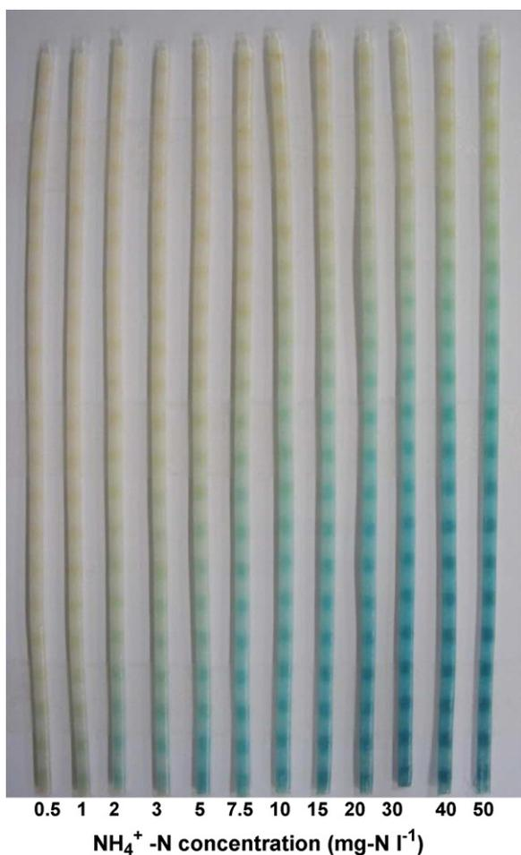
Fig. 4. Zebra-bands formed in detecting tubes.
